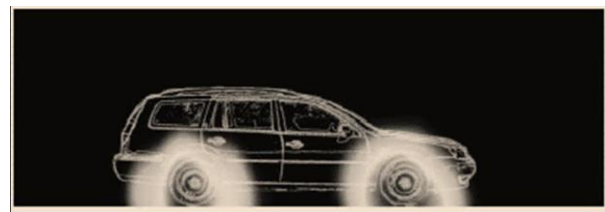
Figure1. Propagation of tyre noise of an automobile at frequency of 600 Hz
